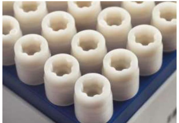
The screw-cap design is suitable for use with an automatic decapper.
