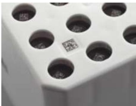
The base of each cryogenic box has a 2D barcode laser etched on to the base. This is used when scanning the tubes, as the Ziath DataPaq™ 2D barcode scanning software uses this extra 2D barcode to determine the orientation of the rack on the scanner bed.
