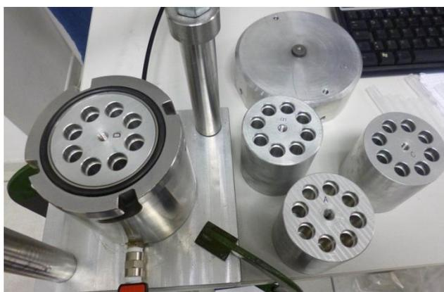
**Figure 1:** To the left the pressure capsule can be seen, with an adapter for a particular tube size inserted. At the back (right) the lid to the pressure capsule can be seen. In front are other adapters for different tube sizes
