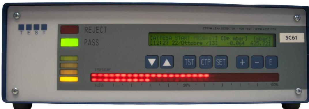
Figure 3: End of Leak Test result. The display shows the date and time of the test, the pressure loss recorded (Dp -0.064mbar) and the pressure at the end of the test (625,721mbar). The green "PASS" light shows the pressure drop value has fallen within acceptable limits (in this case <0.064mbar, maximum pressure drop = 0.2mbar)
