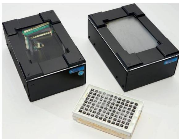
Caption: The scanner on the left has cryoprotection, whereas that on the right uses standard glass. The cold rack has caused a layer of condensate on the untreated glass.
